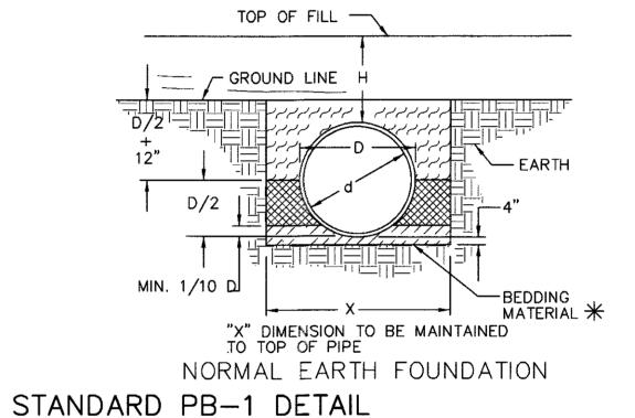
INSTALLATION OF PIPE CULVERTS AND STORM SEWERS CIRCULAR PIPE BEDDING AND BACKFILL METHOD "A" SCALE: NONE
